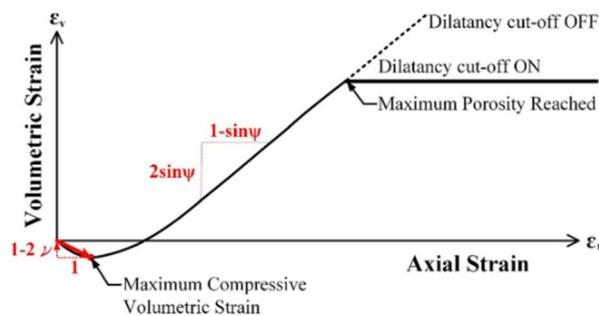
Determination from drained triaxial tests:
